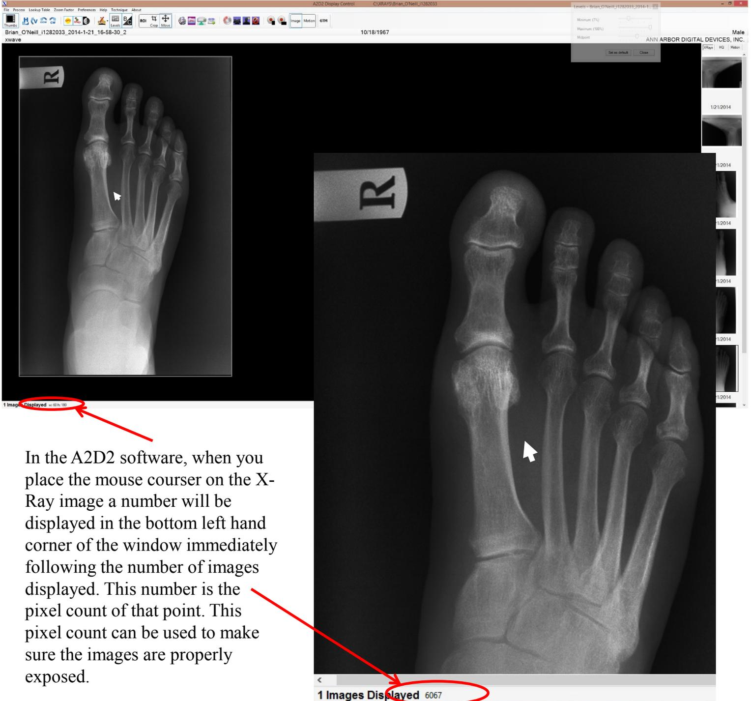
In the A2D2 software, when you place the mouse cursor on the X-Ray image a number will be displayed in the bottom left hand corner of the window immediately following the number of images displayed. This number is the pixel count of that point. This pixel count can be used to make sure the images are properly exposed.
